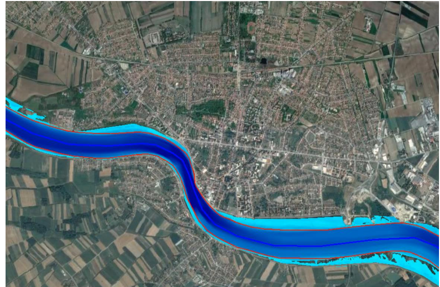
Sava RAS hydraulic model – Levee breach simulation
